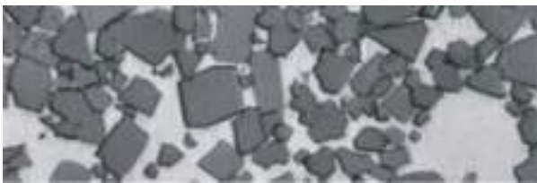
Microstructure of cemented carbide
